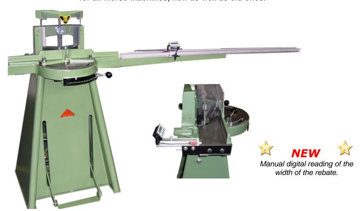
You can now have your new Morso mitring machine delivered with manually operated digital measuring system. This digital measuring system is also available as a subsequent installation on to all existing Morso machines in the market, no matter how old the machine is.
